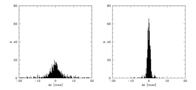
Figure 6: Comparison between isophotal and windowed centroid measurement accuracies on simulated, background noise-limited images. *Left*: histogram of the difference between X\_IMAGE and the simulation centroid in x. *Right*: histogram of the difference between XWIN\_IMAGE and the simulation centroid in x.
