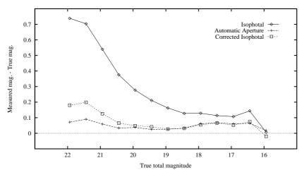
Figure 7: Flux lost (expressed as a mean magnitude difference) with different faint-object photometry techniques as a function of total magnitude (see text). Only isolated galaxies (no blends) of the simulations have been considered.
