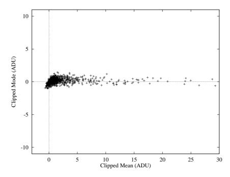
Figure 2: Simulations of  $32 \times 32$  pixels background meshes polluted by random Gaussian profiles. The true background lies at 0 ADU. While being slightly noisier, the clipped "Mode" gives a more robust estimate than a clipped Mean in crowded regions.
