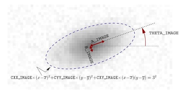
Figure 5: The meaning of basic shape parameters.
