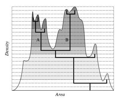
Figure 3: A schematic diagram of the method used to deblend a composite object. The area profile of the object (smooth curve) can be described in a tree-structured way (thick lines). The decision to regard or not a branch as a distinct object is determined according to its relative integrated intensity (tinted area). In that case above, the original object shall split into two components A and B. Remaining pixels are assigned to their most credible "progenitors" afterwards.
