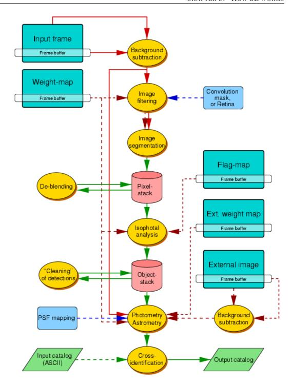
**Figure 5.2:** SE flow diagram from the second manual. This shows clearly the many extra options over a simple run of SE; the possibilities of weight maps, flags, crosscorellation catalogs and many more.
