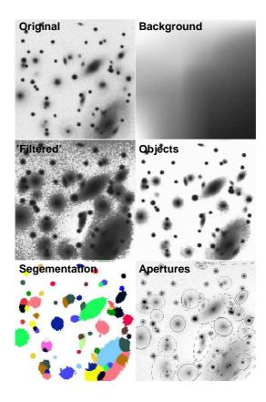
**Figure 7.9:** Illustration of the different checkimages possible. The original inputimage, the BACK-GROUND image, the FILTERED image, the OBJECTS image, the SEGMENTATION image and the APERTURES image. the contrast of the BACKGROUND image has been exaggerated.
