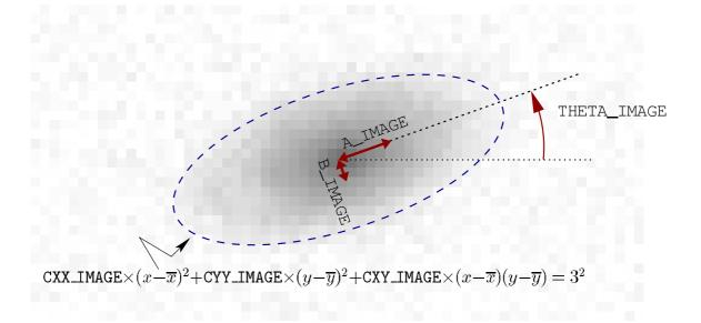
Figure 8.2: Illustration of the Kron radius.  $\bar{x}$  and  $\bar{y}$  are the computed center in of the object.
