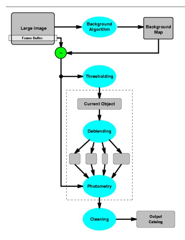
Figure 5.1: SE flow diagram from the first manual. This shows the principal steps done by SE.
