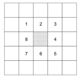
**Figure 7.3:** An object is defined as a series of bordering pixels above the threshold. Bordering pixels to the gray one are 1 through 8. Another pixels needs to be above the threshold and share a corner or a side with another pixel in order to considered part of the same object (unless they are deblended into different objects).
